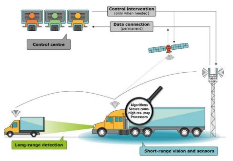
Figure 7: Stylised driverless truck operating environment with optional Control Centre (ITF 2017).
