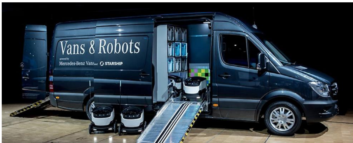
Figure 1: Example of mothership concept where a van serves as hub for up to eight autonomous delivery robots. Source: Daimler https://www.roboticsbusinessreview.com/supply-chain/daimler-invests-robotic-delivery-starship-technologies
