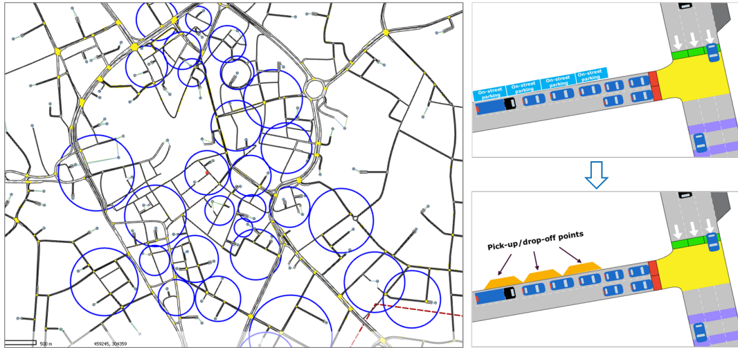
Figure 3.7: Replacing on-street parking with pick-up/drop-off points and the pick-up/drop-off locations in AIMSUN software
